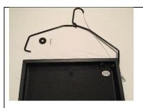
Unlock and open the DOOR, and insert one end of the HANGER into one of the holes in the UNIT (holes on the sides near the top). You can leave the other HANGER end out for now. Place one of the WASHERS on the HANGER end that is inside of the UNIT, then insert the straight leg of the COTTER PIN through the hole in the HANGER end. Pliers may make installation of the COTTER PIN easier.
